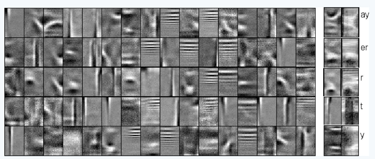
The figure above shows a random subset of features learned in an unsupervised way using a sparse auto-encoder neural network with rectified linear units and natural speech as input. The vertical axis is over frequencies and horizontal axis is over time (26 frames, 10ms long each). The right panel shows examples from the validation set.
